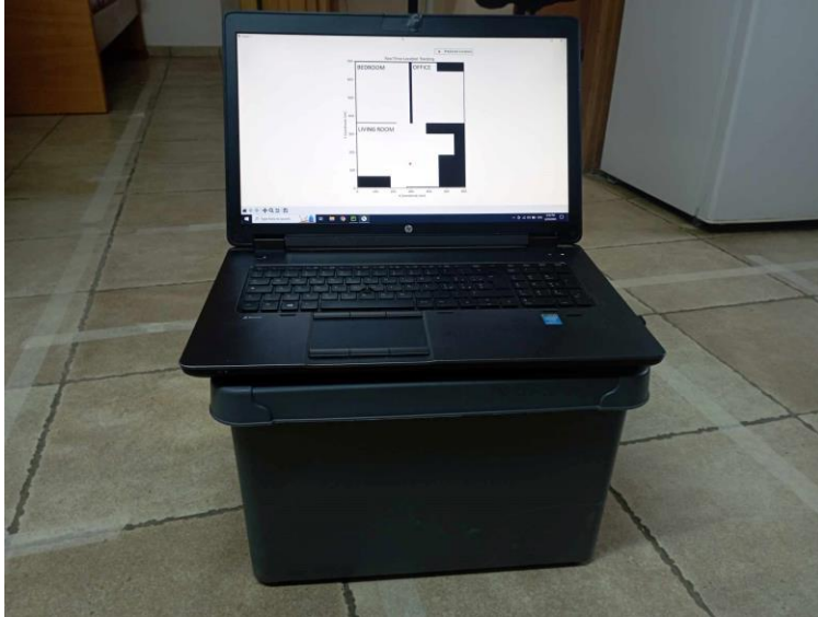
Figure 4: Computer used as mobile robot during the tests. In real robot the computer can be a Raspberry Pi for example.
